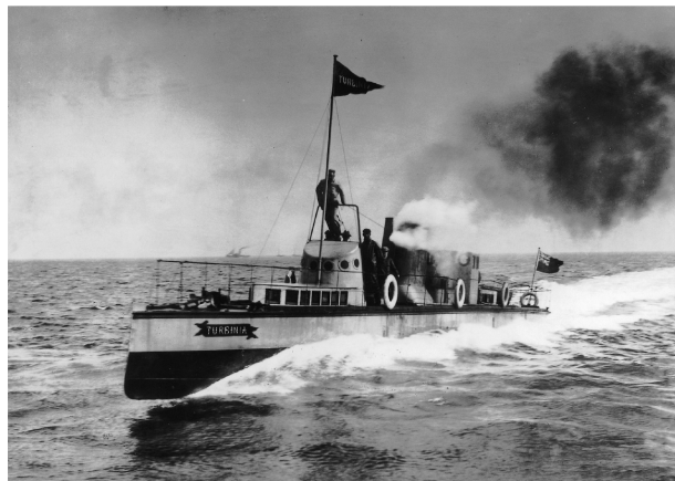
Parsons's ship Turbinia at speed. The turbines drove the ship at over 40 miles per hour.
