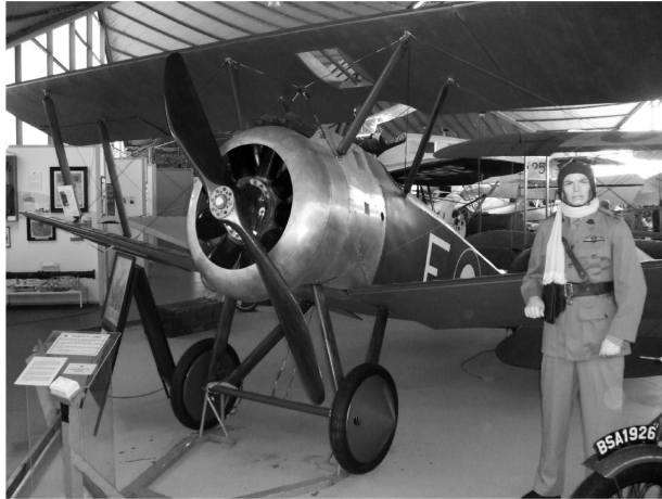
The Sopwith Camel. The propeller is attached to the spinning rotary engine, and the craft's weight is concentrated at the front of the fuselage.
